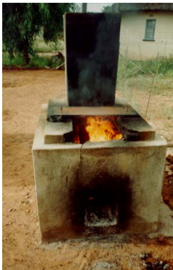
Figure 1: Low technology in-house incinerator
